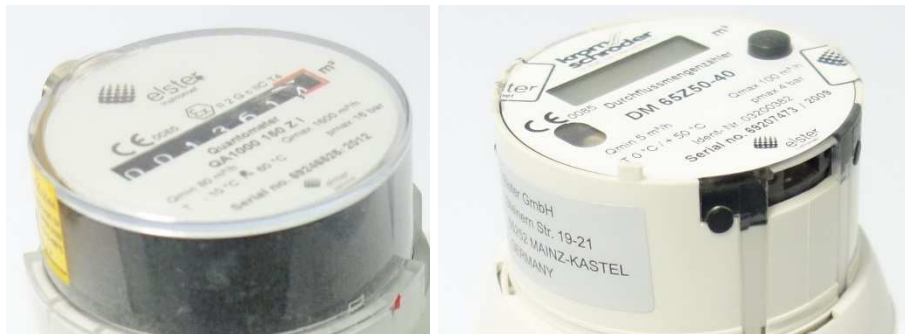
Fig. 2 | Indexes – left: mechanical (QA), right: electronic (QAe)
